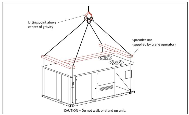
Figure 1. Use a Spreader Bar When Lifting the Rooftop Unit
